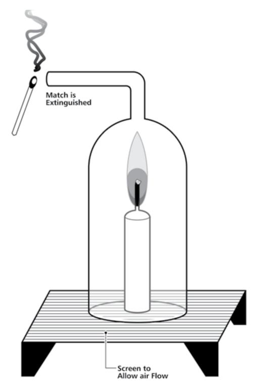
Faraday captures the gases emitted from a candle using a glass jar with a chimney—a glass tube with a right-angle bend. He shows that the flow rate of the gases emitted by the candle are "nearly sufficient to blow" out a match. The match eventually is extinguished because the gases emitted by the candle—including  $CO_2$ , and  $H_2O$ , which are produced by the chemical reaction in the flame, plus  $N_2$ that entered as part of the incoming air—will not sustain combustion.
