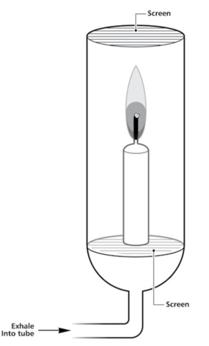
Faraday uses this apparatus to demonstrate that gases humans exhale won't sustain combustion. He breathes gently into the lower tube, so that his breath won't blow out the candle directly. As the exhaled gases surround the flame, it flickers and then goes out. Faraday shows later in this lecture that these exhaled gases contain  $CO_2$  like the gases emitted by a candle.
