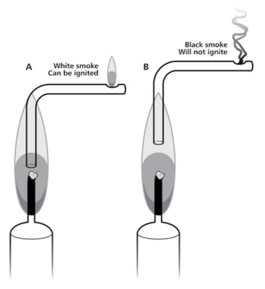
Faraday uses a glass tube with a right-angle bend to probe the flame. **a** The white smoke produced near the tip of the wick contains vaporized wax and can travel through the pipe and be lit. **b** The black smoke produced near the middle of the flame cannot be lit.
