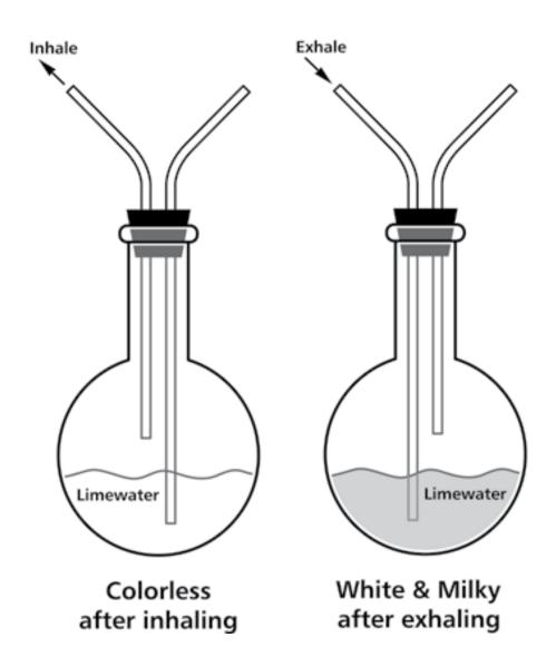
Faraday uses this apparatus to show that human breath contains  $CO_2$ . **a** Faraday draws in a breath through the limewater: he observes no change in the limewater. **b** He rotates the apparatus and exhales into the limewater: it now turns cloudy. Limewater turns cloudy, as he showed in an earlier lecture, when  $CO_2$  gas is bubbled through it.
