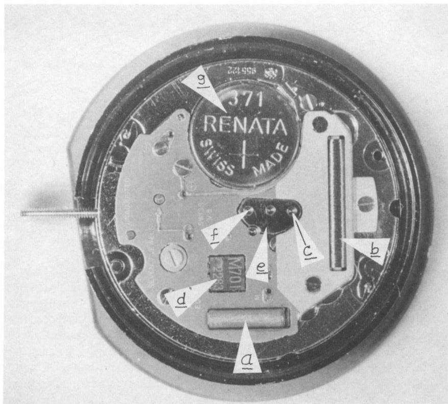
**Fig. 1.** Quartz analog watch with back cover removed. **a**, capsule that contains the quartz tuning fork; **b**, coil that momentarily magnetizes the stator of the motor; **c**, axle of the motor armature; **d**, integrated circuit (IC); **e**, gear box; **f**, concentric axles of the three hands; **g**, battery.
