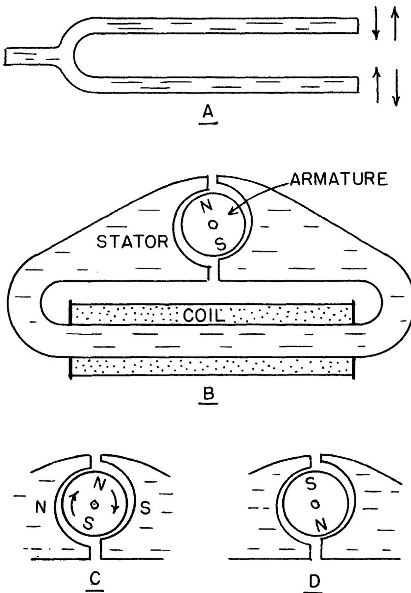
Fig. 2. **A**, a conventional tuning fork; vibrates the same way as the one in the watch. **B**, the motor, with the armature in the resting position when the stator is unmagnetized. **C**, current in the coil, stator magnetized in the sense shown, armature starting rotation, clockwise. **D**, stator again unmagnetized, armature comes to rest as shown, 180 degrees from starting position.
